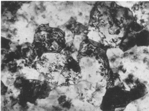
Figure 7 Recovery structures in SAP 5.25 wt % oxide annealed 1800 sec at 380° C ( \times 18000 ).
