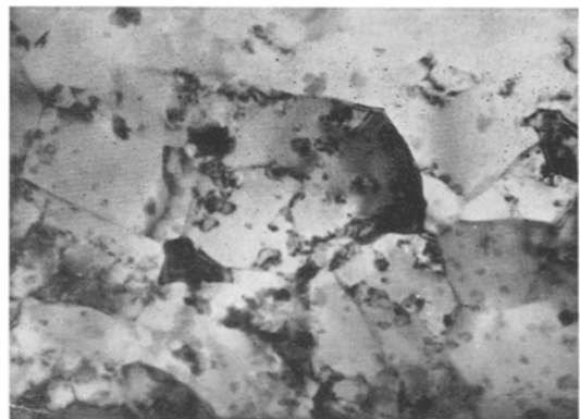
Figures 4, 5 Structural features of the unrecrystallised portions of SAP 5.25 wt % oxide specimens, heated at 480°C. (4) After 10 sec heating; (5) after 3600 sec ( \times 18000 ).
