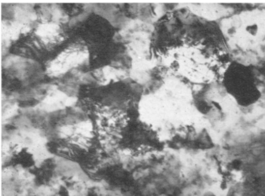
Figures 4, 5 Structural features of the unrecrystallised portions of SAP 5.25 wt % oxide specimens, heated at 480°C. (4) After 10 sec heating; (5) after 3600 sec ( \times 18000 ).
